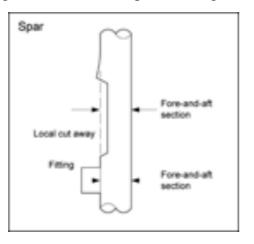
H.4.2 Fittings, local curvature and local cut away, shall be ignored when measuring a spar or dimensions taken to a spar.
